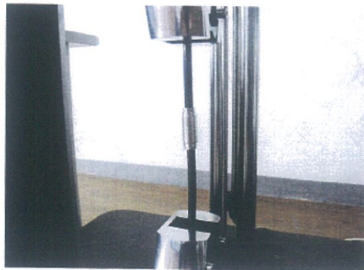
Picture 04: Pull-off strength
